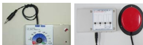
(a) (b) Fig. 1 Developed AT apparatus. (a) Switch Latch and Timer (b) Switch IR learning remote controller
