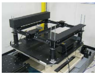
Fig. 1 Isolation test specimen on shaking table.
